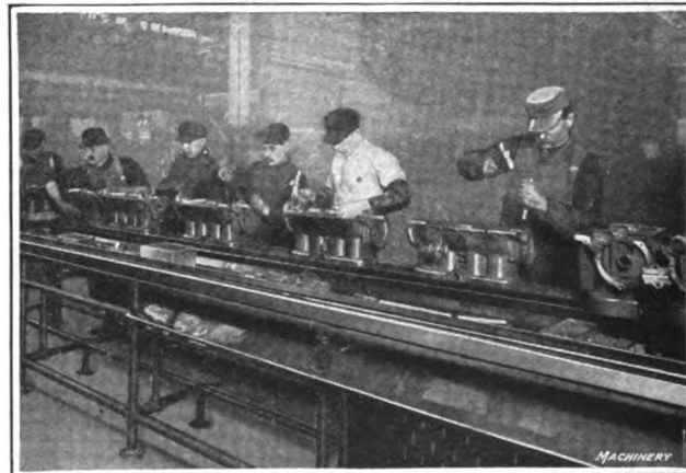
Fig. 25—In the Ford Motor Co.'s plant every possible saving is effected in production. In assembling motors, as fast as one man finishes his task he pushes the motor along to his companion and receives a new motor from the man on the other side. This is another example of the progressive method of assembling
